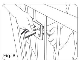
First, place one clamp plate (Item 1) on the side of the railing you want to place the Orbis. Then slot the M8 x 80mm screw (Item 3) through the four inner most holes of it, through the railings. Next, position the other clamp plate and slot 4 M8 x 35mm screws (Item 2) through the outer holes of both clamp plates (Item 1), (See Fig A.) When all the screws and plates are lined up tighten the outer screws using 4 M8 x 20mm washers (Item 4), 4
